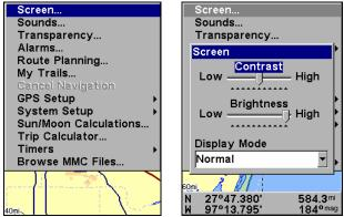
Screen selected on main menu (left). Screen Menu with Contrast bar selected (right). To adjust the display's brightness:
